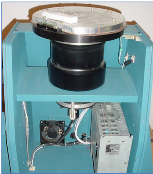
Figure 93: A typical rate table used for tuning gyros. (Ideal Aerosmith, Inc)
