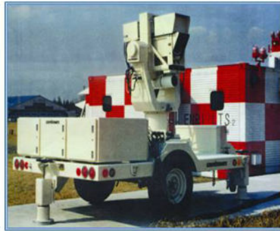
Figure 123: A mobile laser missile-tracking system. (Contraves)
