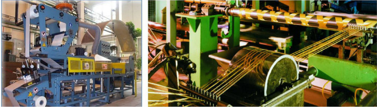
Figure 64: Left: A prepreg machine constructed by the Composite Materials Group for the production of prepreg materials using fibers and resins. (Katholieke Universiteit Leuven) Right: A machine adding resin to seven lines of roving. (Hunting Engineering, Ltd.)
