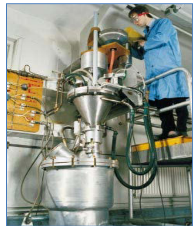
Figure 51: Slurry cast double-base mixing equipment for small motor. (British Aerospace Limited)
