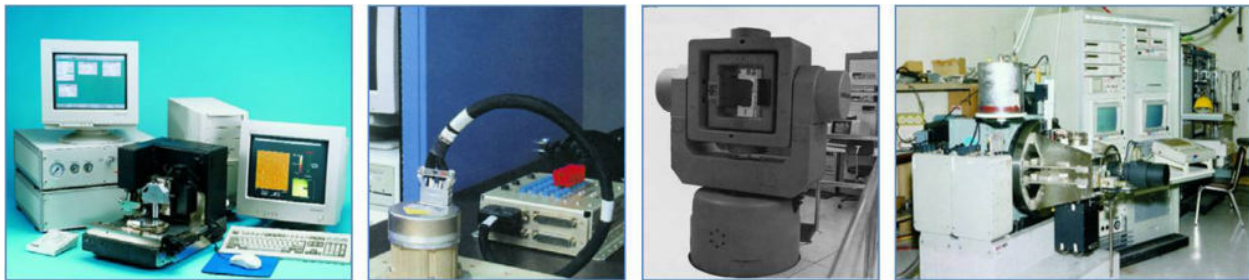
Figure 95: Left : a profilometer system used for measuring mirrors. (Digital Instruments) Middle left : is another portable IMU tester connected to a miniature IMU. (Litton Guidance and Control Systems) Middle right : is a three-axis table for testing IMUs or gyros.
