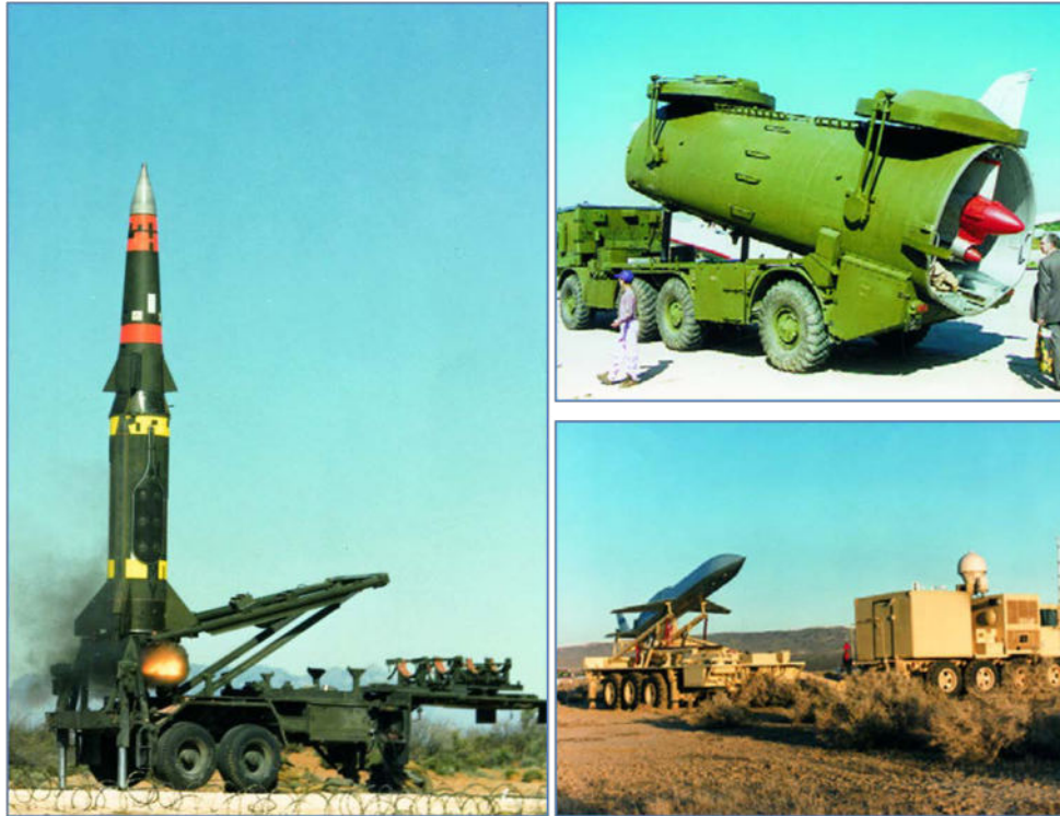
Figure 113: Left : an erector launcher detached from its prime mover. (MTCR Equipment, Software and Technology Annex Handbook, Third Edition (May 2005)). Top right : a transporter erector launcher for a large, Category II cruise missile. (MTCR Equipment, Software and Technology Handbook Third Addition (May 2005)). Bottom Right : Erector launcher for a rocket-assisted UAV and its associated command-and-control van. (Teledyne Ryan Aeronautical)
