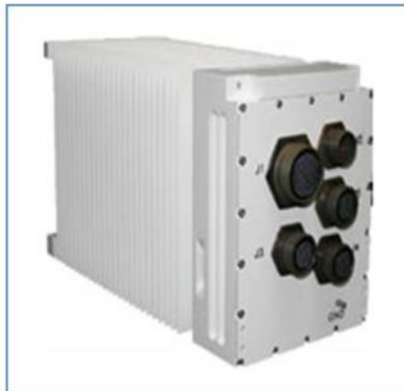
Figure 128: Another mission computer for multiple platforms, this one is designed for use in harsh aerospace and military applications. (Curtiss Wright Embedded Computing Controls)
