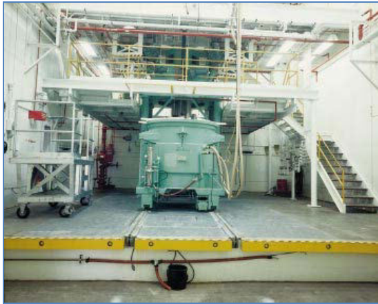
Figure 52: A 420-gallon propellant mixing bowl. (ATK)
