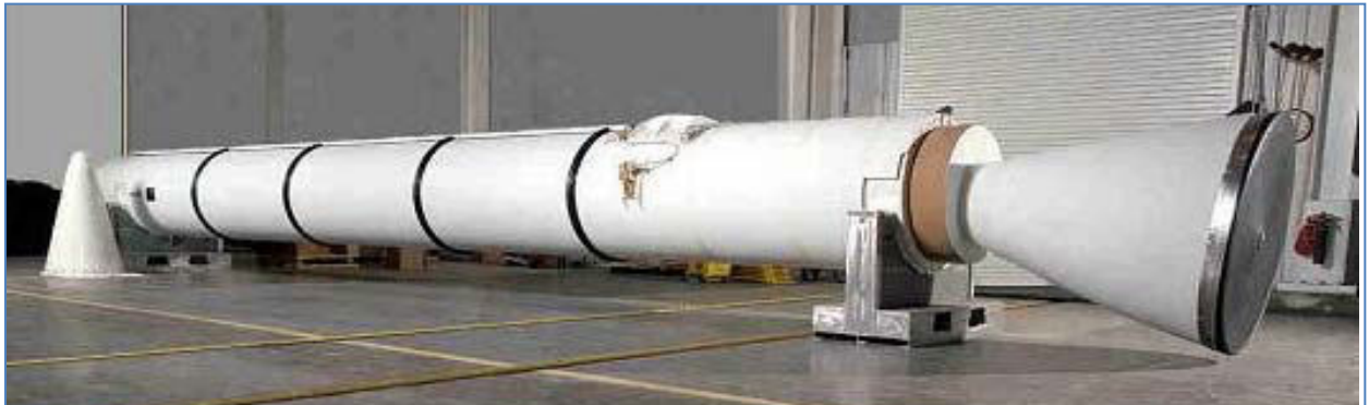
Figure 35: A rocket motor with a large fixed, canted nozzle. The motor is used on a launch vehicle. (ATK)
