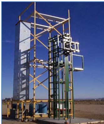
Figure 141: A vertical test stand designed for testing liquid propulsion rocket engines. (Interorbital Systems)
