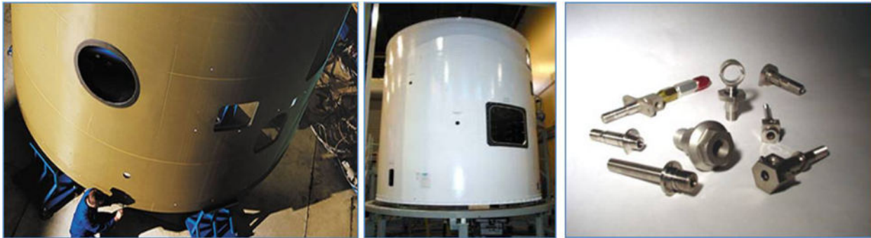
Figure 37: Left: A large composite center-body section designed for a space launch vehicle. (ATK) Center: A typical rocket interstage section. (ATK) Right: A selection of explosive bolts designed for use in space launch vehicles and military applications
