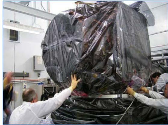
Figure 132: Vibration testing of a laser altimeter system. (NASA)
