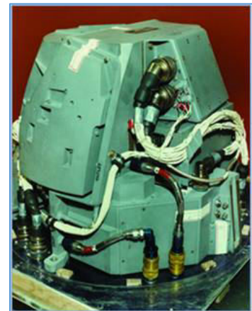
Figure 74: The main body of a cruise missile's integrated flight instrument system. (Litton Guidance and Control Systems)
