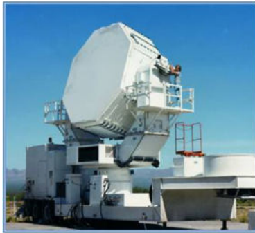
Figure 124: A mobile phased-array missile tracking radar. (MTCR Equipment, Software and Technology Annex Handbook, Third Edition (May 2005))
