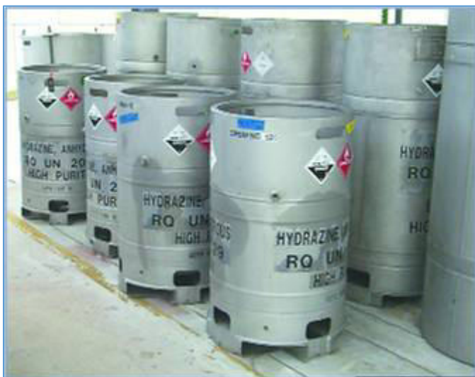
Figure 57: 34-gallon anhydrous hydrazine shipping containers made of 300-series stainless steel. (MTCR Equipment, Software and Technology Annex Handbook, Third Edition (May 2005))
