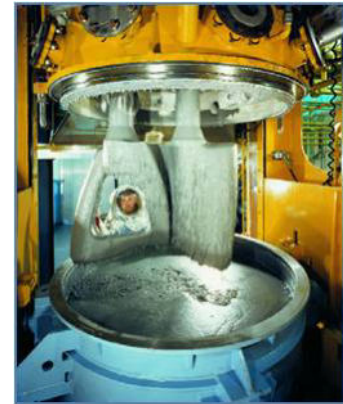
Figure 53: Solid propellant being mixed in a 600-gallon vertical planetary mixer. (Thiokol Corp.)
