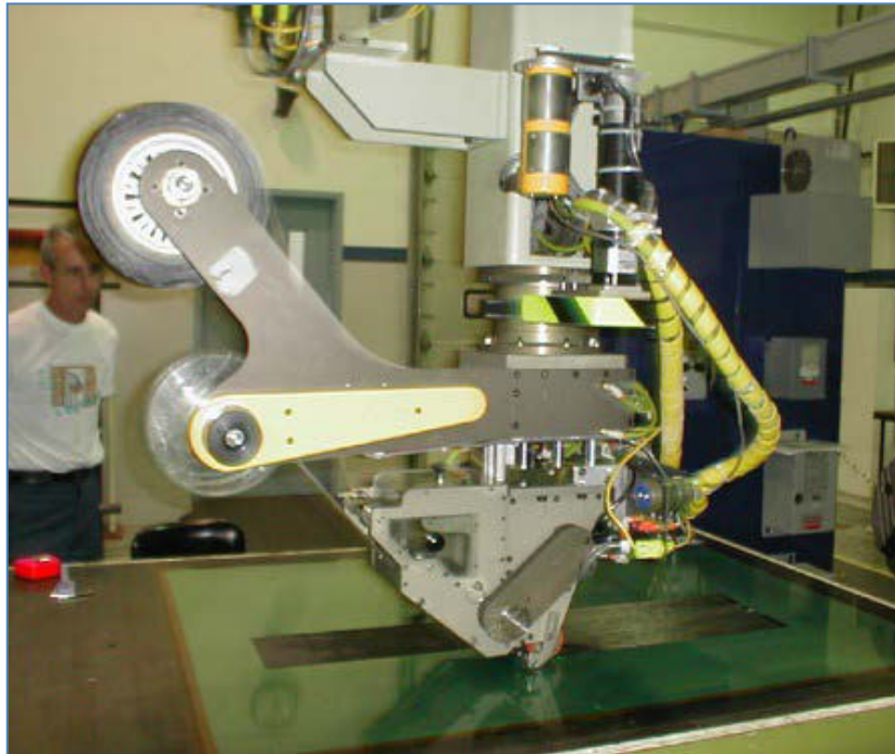
Figure 62: An automated tape-laying machine head. (Automated Dynamics)
