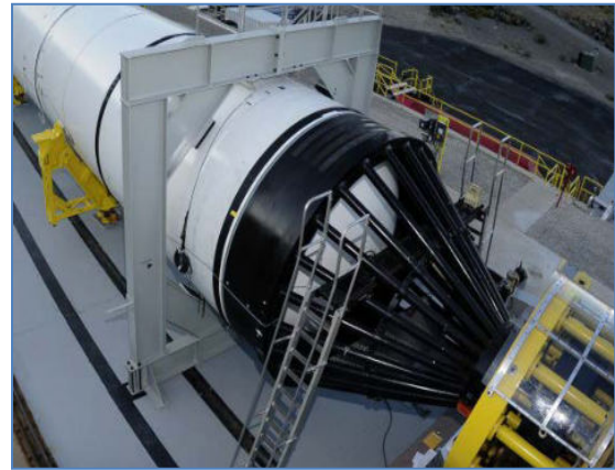
Figure 139: The load measurement system on the test stand of a solid rocket motor. (ATK)
