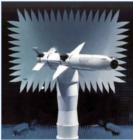
Figure 156: A target missile in the Bistatic Anechoic Chamber (BAC) RCS measurement compact range. (U.S. Navy)
