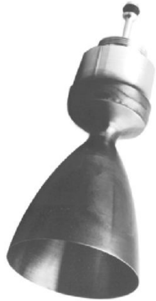
Figure 46: A small rocket thruster that uses liquid hydrazine monopropellant. The thrust chamber wall is thin metal without cooling passageways, so the surfaces are darkened in color due to high temperatures. The bright metal portion remains cooler due to liquid flow through the injector. Overall length is approximately 0.1 m. (Aerojet Redmond and Lawrence Livermore National Laboratory)
