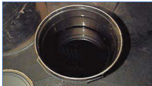
Figure 59: A Polybutadiene-Acrylic Acid-Acrylonitrile (PBAN) shipping drum. (The Charles Stark Draper Laboratories)
