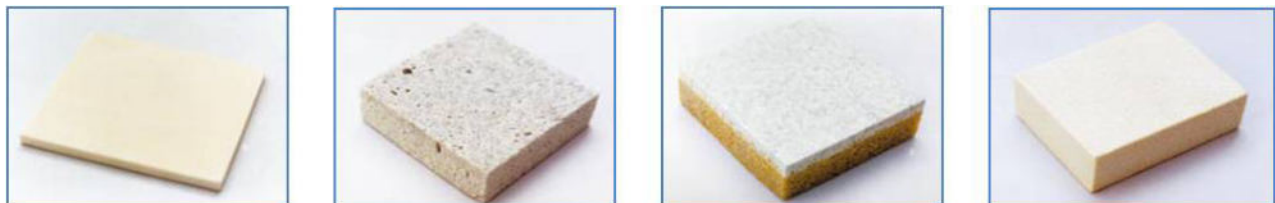
Figure 153: Four radar absorbing material foams, from left: low-dielectric foam (epoxy); lightweight lossy foam (urethane); sprayable lightweight foam (urethane); and thermoplastic foam (polytherimide). (MTCR Equipment, Software and Technology Annex Handbook, Third Edition (May 2005))
