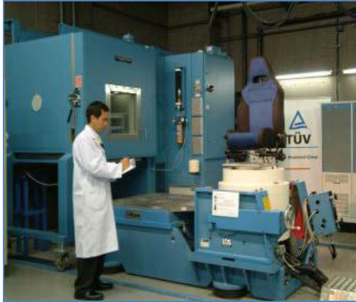
Figure 143: A vibration and environmental test apparatus configuration. (TUV Rheinland)
