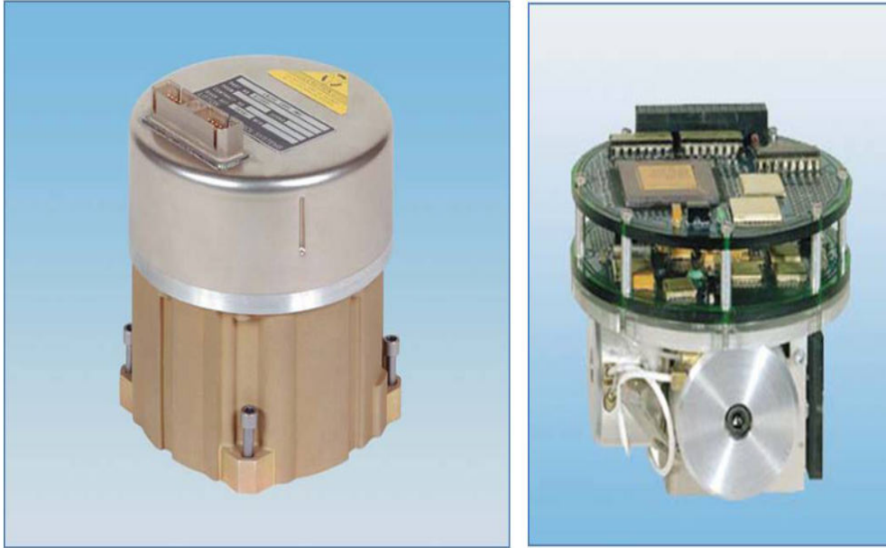
Figure 87: An Inertial Measurement Unit (IMU) utilizes inertial fiber optic gyros (FOGs) and micro-machined accelerometers and is used in space stabilization, missile guidance, UAV guidance and flight control. (Northrop Grumman)
