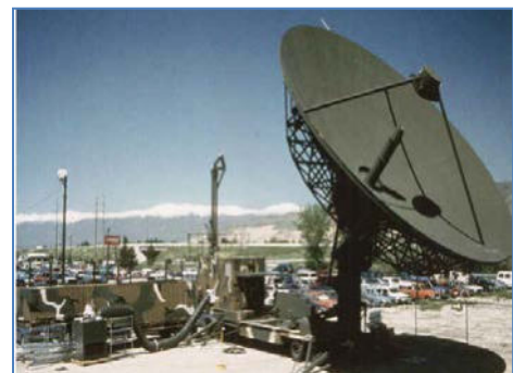
Figure 119: A large SATCOM military antenna designed for major command posts and mobile command posts, and suitable for communications with UAVs. (General Dynamics)
