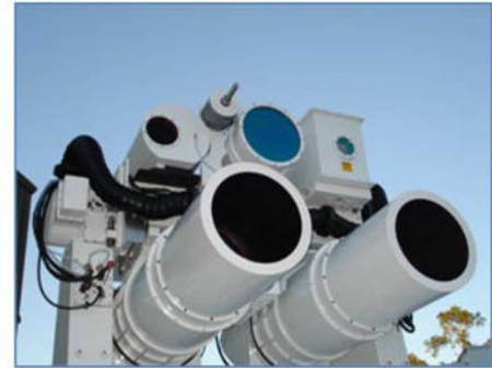
Figure 122: An electro-optical laser tracking system. (BAE Systems)
