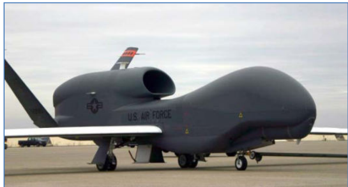
Figure 5: A High Altitude Long Endurance (HALE) Unmanned Aerial Vehicle (UAV). (U.S. Air Force)
