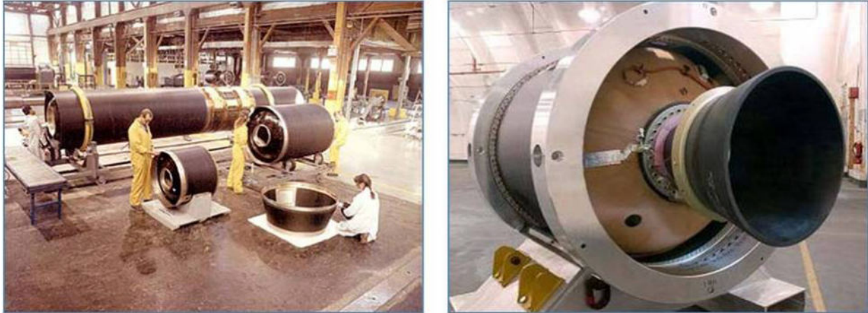
Figure 33: Left: A selection of composite rocket motor cases designed to support a range of mission platforms, including the first, second and third stage rocket stages of a space launch vehicle. (ATK) Right: A rocket motor – installed in a case – which functions as the third-stage of a launch vehicle. (ATK)
