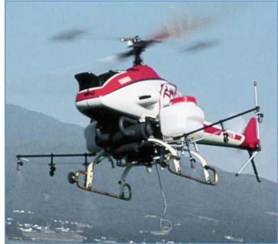
Figure 166: A rotary-wing UAV designed with chemical tanks and spraybars for agricultural purposes. (Yamaha)
