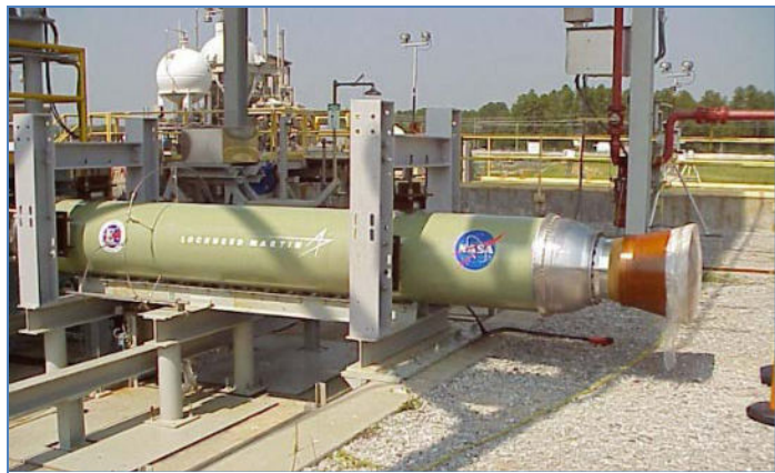
Figure 41: A hybrid sounding rocket motor. (NASA)
