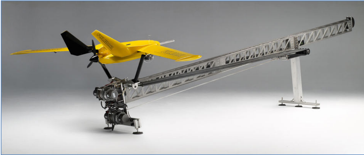
Figure 164: A medium-range endurance UAV. Despite its small size, this elastic catapault-launched UAV is capable of carrying a 1 kg payload (IR and digital cameras) to a range of 400 km. (Aerovision Vehiculos Aereos, SL)
