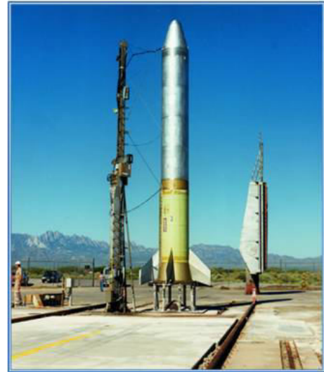
Figure 108: Minimal launch pad with a gantry and connections to a complete rocket system. (MTCR Equipment, Software and Technology Annex Handbook, Third Edition (May 2005))
