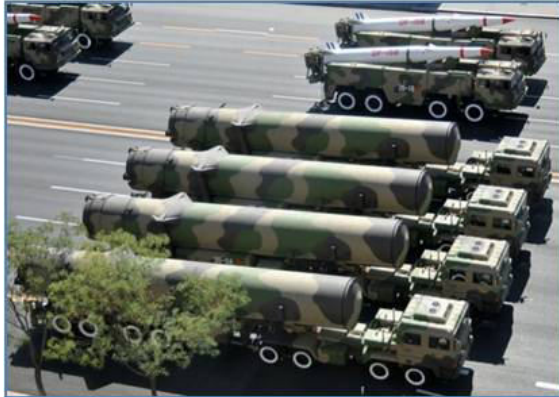
Figure 111: Above: Eight axle TELs carrying intercontinental ballistic missiles (ICBMs; foreground) and four axle TELs carrying intermediate range ballistic missiles (IRBMs). (Via Chinese Internet)
