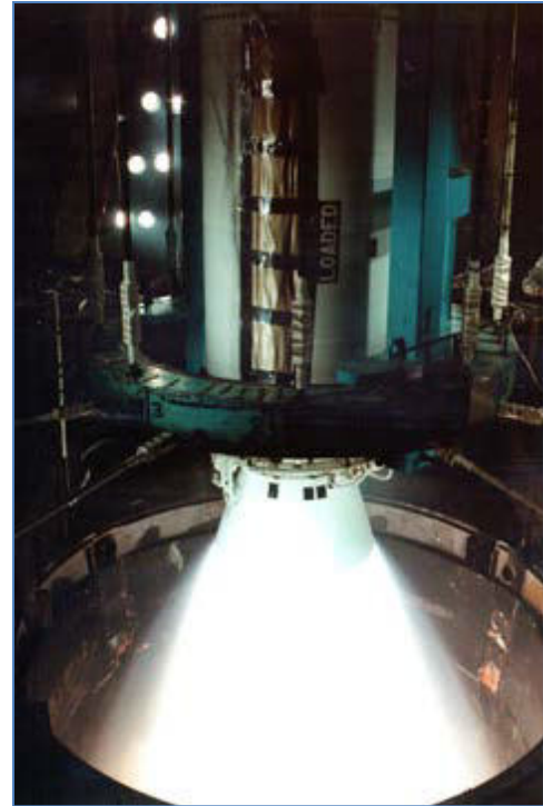
Figure 142: A full scale solid rocket engine being tested at simulated high altitude. (AEDC)
