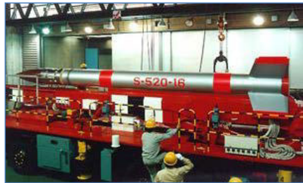
Figure 162: A large Category II sounding rocket, capable of delivering a 250 kg payload to a range of 400 km. The rocket's solid propellant motor, with steel casing, is surrounded by four honeycomb tail fins with titanium alloy leading edges. (JAXA)
