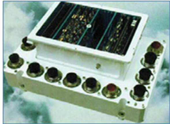
Figure 104: Digital signal processor with the lid removed. The size is 5 cm to 7.5 cm on each side. (MTCR Equipment, Software and Technology Annex Handbook, Third Edition (May 2005))
