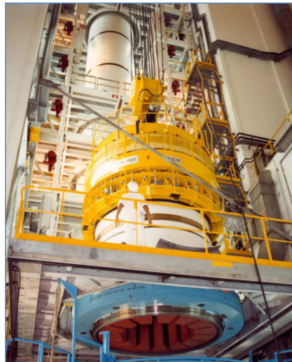
Figure 12: Solid propellant rocket motor stage being positioned onto a space launch vehicle (above). (European Space Agency)
