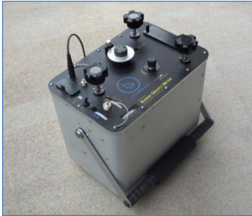
Figure 115: This automated gravity meter is one of the most precise, rugged and lightweight gravity meters. Under normal conditions, it can be leveled for mGal readings within 30 seconds, and has a drift rate of less than 0.5 mGals per month. (ZLS Corporation)
