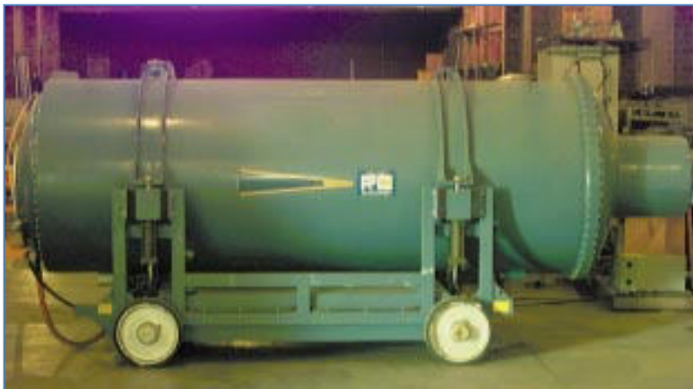
Figure 146: A 2.3MeV flash X-ray unit used for inspecting solid rocket motors. (MTCR Equipment, Software and Technology Annex Handbook, Third Edition (May 2005))
