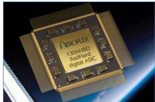
Figure 158: A radiation hardened application specific integrated circuit (ASIC) designed for high reliability and radiation-intense applications. (Aeroflex)
