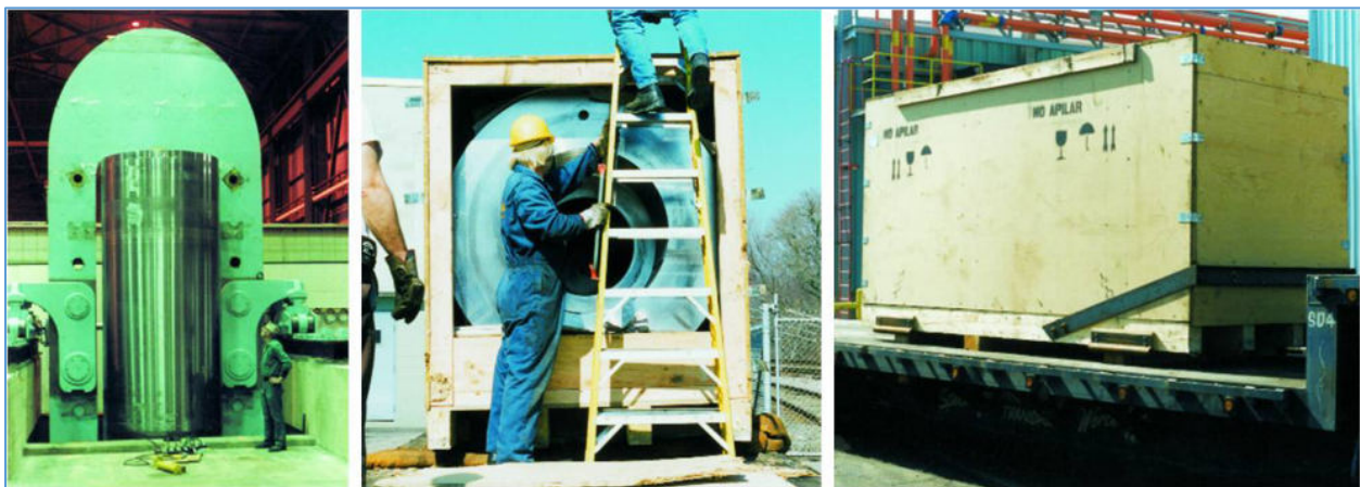
Figure 66: Left: Side view of a large isostatic press. (Engineered Pressure Systems, Inc.) Center and Right: Two different views of an alternative shipping crate for an isostatic press. (Engineered Pressure Systems, Inc.)
