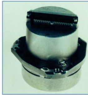
Figure 82: A dynamically tuned gyro (DTG). (The Charles Stark Draper Laboratories, Inc.)
