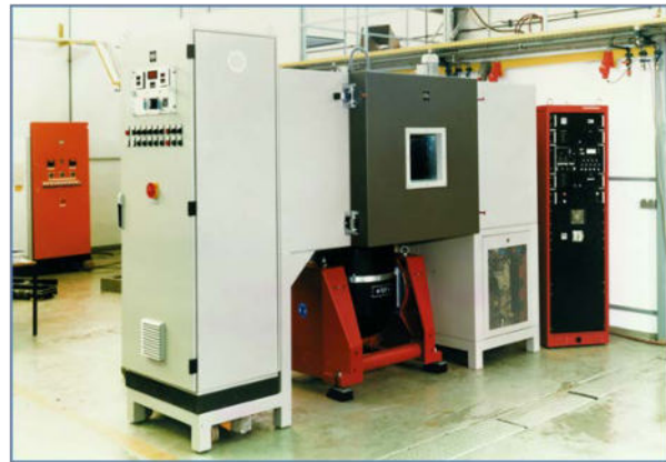
Figure 144: A controlled environmental chamber with vibration capability. (RMS Dynamic Test Systems)
