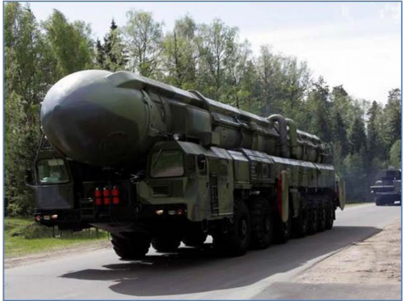
Figure 3: Left: A Space Launch Vehicle (ISRO). Right: Road Mobile SS-25, a solid propellant, single warhead intercontinental ballistic missile (ICBM). (Maxim Shipenkov/AFP/Getty Images)
