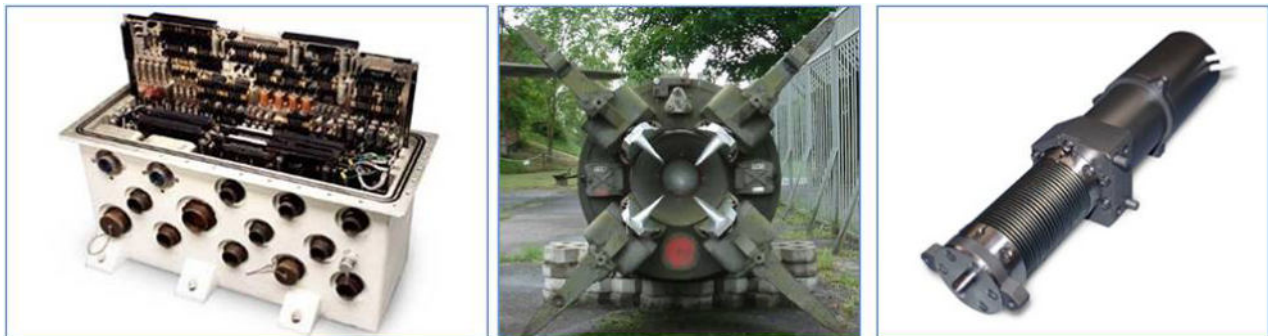
Figure 23: Left: A thrust vector control electronics box for use in large launch vehicle applications. (Moog, Inc.) Center: Four jet vanes mounted in the rear of a ballistic missile. (Russian military) Right: A fine positioning linear actuator designed for use in space applications. (Moog, Inc)
