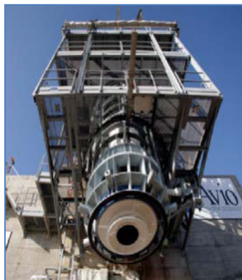
Figure 140: A solid propellant rocket motor on a test stand. (Avio SpA)
