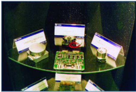
Figure 83: A FOG (left), an RLG (center), and an accelerometer (right). (MTCR Equipment, Software and Technology Annex Handbook, Third Edition (May 2005))
