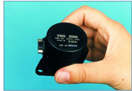
Figure 81: A vibrating structure gyro. (British Aerospace Ltd.)
