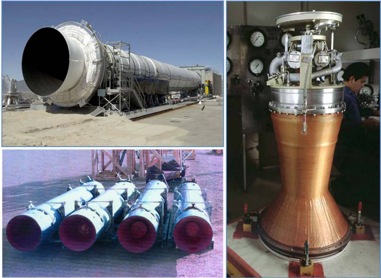
Figure 18: Top left: A re-usable solid rocket motor for space vehicle use. (ATK) Bottom left: Solid propellant rocket motors with total impulse close to the lower limit of Item 2 control. (MTCR Equipment, Software and Technology Handbook, Third edition (May 2005)) Right: A pressure-fed liquid rocket engine. (Aerojet)
