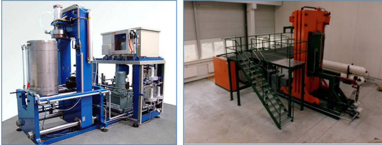
Figure 65: Left: A laboratory sized isostatic press. (ESPI) Right: A laboratory sized hot isostatic press. (Abra Fluid AG)
