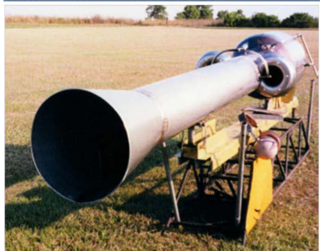
Figure 30: Top: A large ramjet engine. (March Field Air Museum) Middle: A scramjet engine completes a Mach 5 test at a wind tunnel facility. (Pratt & Whitney / NASA) Bottom: A modern pulsejet engine with a rearward facing intake. (Thermojet)
