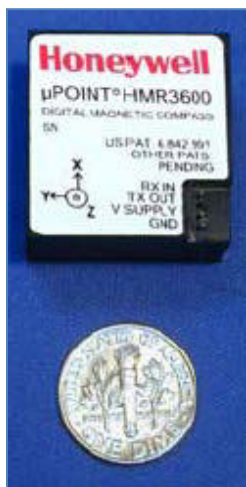
Figure 92: This gyro-stabilized magnetic compass module uses three-axis magnetic heading sensors. (Honeywell)
