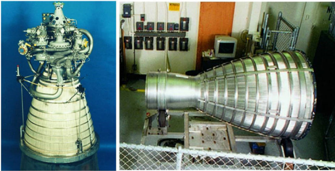
Figure 45: Top left: A liquid rocket engine with a large, regeneratively cooled nozzle. (MTCR Equipment, Software and Technology Handbook, Third edition (May 2005)) Bottom right: Side view of a regeneratively cooled liquid rocket nozzle, joined to its combustion
