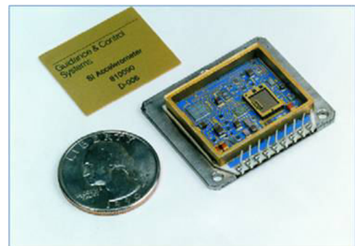
Figure 86: An integrated circuit accelerometer rated at over 100 g. (MTCR Equipment, Software and Technology Annex Handbook, Third Edition (May 2005))
