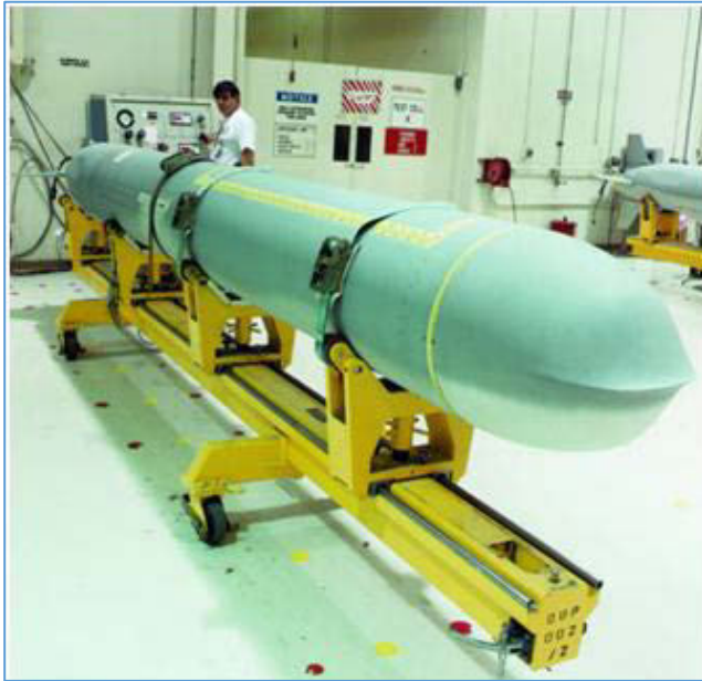
Figure 7: An operational cruise missile on its checkout stand, showing its nose cone modified to lower radar returns and enhance aerodynamic performance. (MTCR Equipment, Software and Technology Handbook, Third edition (May 2005))
