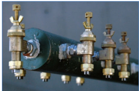
Figure 165: A Modular Aerial Spray System, used for pesticide application, can use a setting called ultra-low volume and specialized spray boom nozzles such as those shown here to spread one half to an ounce of chemical over an acre. (U.S. Air Force)
