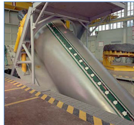
Figure 49: Solid propellant in liquid form is poured into rocket casings and cast into the required shape. The casting is moved by a hydraulic mount to remove bubbles or other defects. (ATK)
