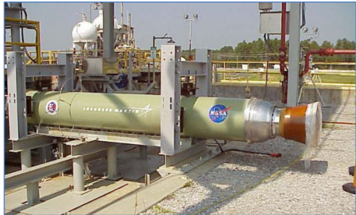
Figure 19: A hybrid sounding rocket motor. (NASA)
