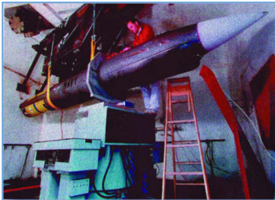
Figure 133: A thruster being prepared to vibration-test a missile. (Unholtz-Dickie)
