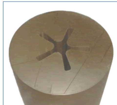
Figure 56: A sample of double-base rocket motor propellant. (Bayern-Chemie GmbH)
