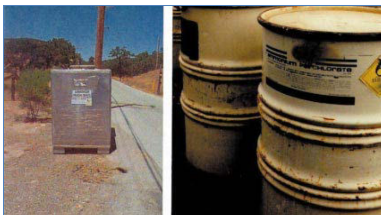
Figure 58: Two different ammonium perchlorate shipping containers. (The Charles Stark Draper Laboratories & Kerr McGee)
