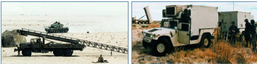
Figure 114: A pneumatic UAV launcher. Right: Command-and-control vehicles suitable for launching missiles from fixed or mobile locations. (MTCR Equipment, Software and Technology Annex Handbook, Third Edition (May 2005))
