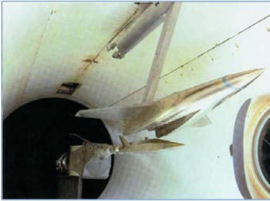
Figure 138: Test objects in test section of a hypersonic wind tunnel. (MTCR Equipment, Software and Technology Annex Handbook, Third Edition (May 2005))
