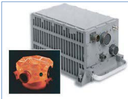
Figure 89: An internal Inertial Measurement Unit (IMU) and GPS with laser gyro (inset). (Northrop Grumman)
